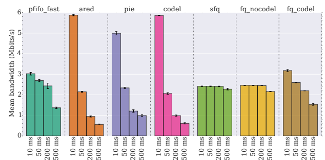
Figure 2: RTT fairness results. The graphs show the aggregate mean goodput of each of the four TCP flows for each queue management scheme.
